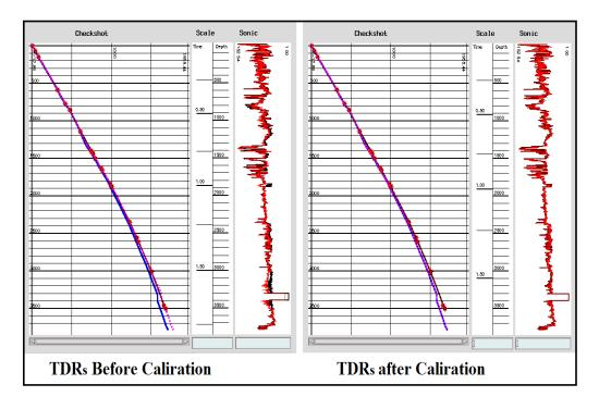
Figure-2. The calibration processes by time-depth relation of sonic and check-shots curves in Samawa-1 well.
