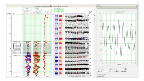
Figure 14. Well-Seismic Correlation, blue is the synthetic; red is trace around the well.
