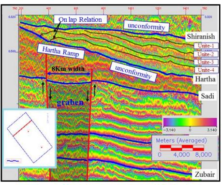
Figure-7.An instantaneous phase section inline no. 45375 shows Shiranish Progradational mound (on-lap relation sequence).
