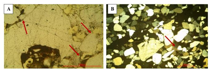
Plate 8. A. Clay Cement. Kf-1 (2010m) B. Calcite Cement. Kf-1 (2200m)
