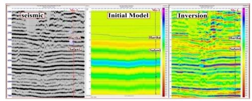
Figure 15. Shows seismic section, low frequency initial model LFM and inverted section matching well logs.
