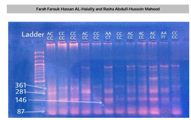
Figure 1 : Agarose gel electrophoresis showing the detection of two *MTHFR*gene polymorphism (C677Tand A1298C) by tetra-primer ARMS-PCR.
