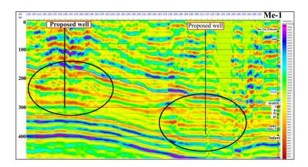
Figure 17. Acoustic impedance (AI) section shows a low AI throughout the entire interval of mound in the Hartha formation, which indicated a high porosity.
