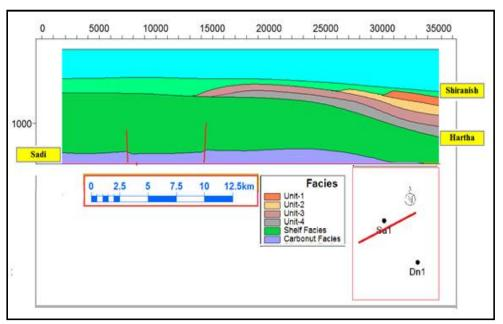
Figure-18.Reflection streangth attribute section shows high negtive of amplitude values at unite-3 of Shiranish Fn.
