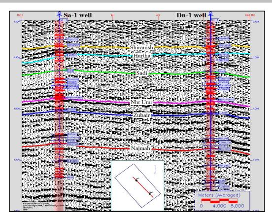
Figure-5.An arbitrary seismic section shows seismic correlation of picked reflectors between synthetic traces of Sa-1 and Dn-1 wells.
