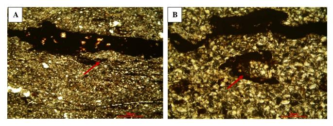
Plate 9.A & B Dissolution in shale unit of Zubair Formation.Kf-3 (2350m)
