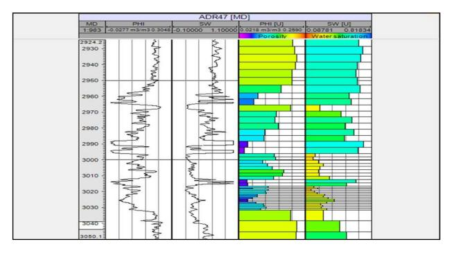
Figure 7. Scale up of porosity and water saturation for well ADR47
