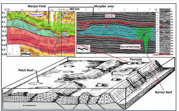
Figure 5.Illustrates distribution of the reef types and seismic sections show the pinnacle reef seismic facies in the Merjan and the barrier reefseismicfacies companied with karst and fluid leakage in the Musyibe area.
