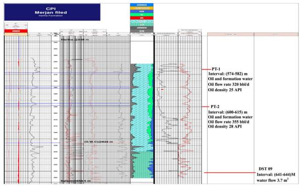
Figure 8. Computer Processed Interpretation (CPI) showing a hydrocarbon charged reservoir of Hartha formation in the Me-1 well.
