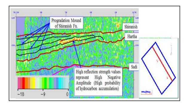
Figure-17.Lithofacies dip section derived from a seismic interpretation and wells data in the study area.
