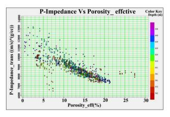
Figure 16. P-impedance versus porosity cross plot from Hartha to Safawi formation.
