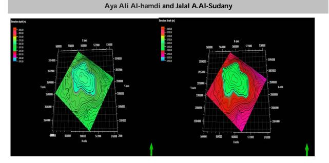
Figure 3. 3D structural modeling of two units fromRumailareservoir in Ahdedoil field.
