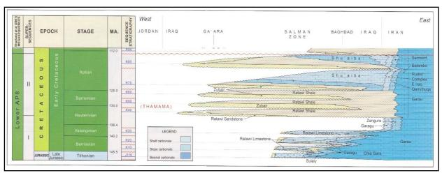
Figure 2. Schematic west-east profile across Southern/ Central Iraq illustrating stratigraphic position of Zubair Formation (Aqrawi, et al. 2010)
