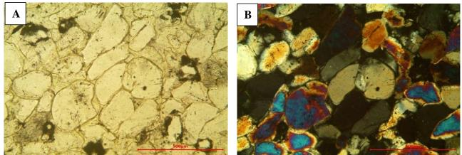
Plat (6) A. Quartz overgrowths.Kf-1 (2200m) B. Quartz overgrowths under the polarized.Kf-1 (2450m)
