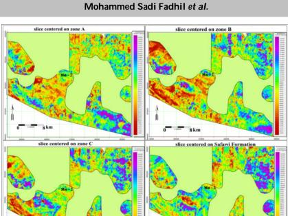
Figure 18. AI inverted Time slice distributed vertically through the reservoir of Hartha to Safawi formation.
