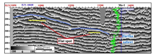
Figure 11. 3-D In-line instantaneous phase section shows flat spot features through mound seismic facies in the Hartha formation.
