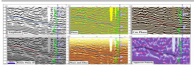
Figure 9. 3-D seismic attributes sections through mound seismic facies in the Hartha formation.
