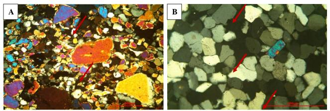
Plat (4) A & B Chemical compaction, point – contacts evolve through straight – elongate to concave – convex and even sutured contacts.A. Kf-1 (2450) B. Kf-1(2200m).
