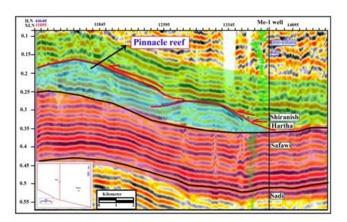
Figure 3. Seismic section show mound seismic facies which indicates biohermal shape in the Hartha formation.
