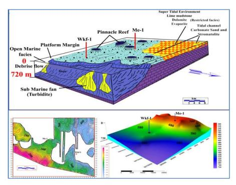
Figure 4. Model of facies distribution of Hartha carbonate buildup and two way time map of mound feature.
