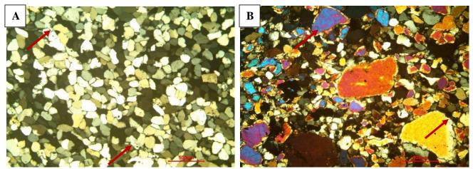
Plat (7) A & B Micro Crystalline Quartz cement.A.Kf-1 (2090m) B.Kf-1(2450m).
