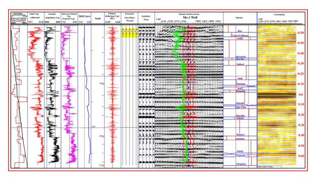
Figure 2.Synthetics seismogram of Me-1 which shows a good tie with seismic data.
