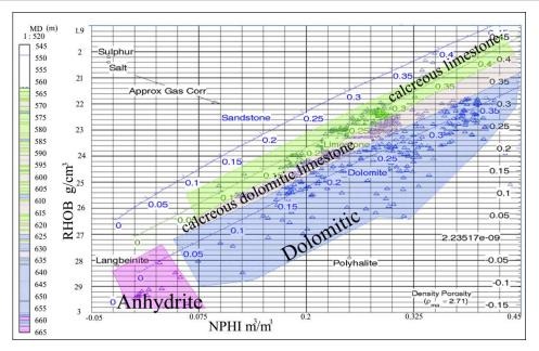
Figure 7. Neutron–Density Cross-Plot illustrates the Lithology distribution of Hartha formation in well Me-1
