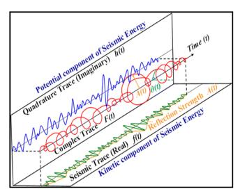
Figure-6. The complex seismic trace and seismic attributes.
