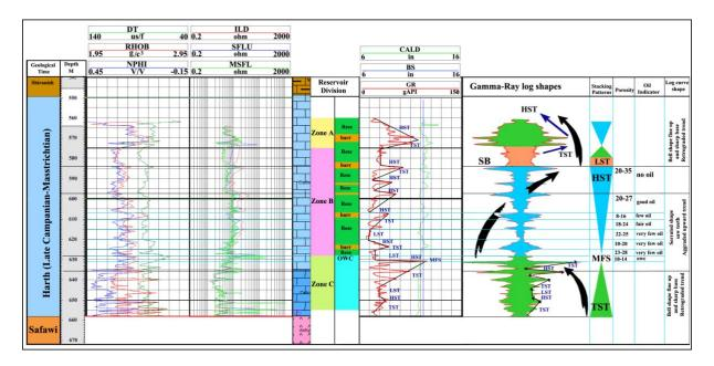
Figure 6.Sequence stratigraphic section and reservoir division of Hartha formation of the Me-1 well.
