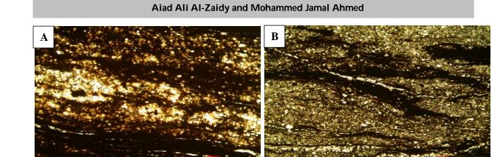
Plat (5) A & B shale compaction in Zubair Formation.Kf-3 (2350m).
