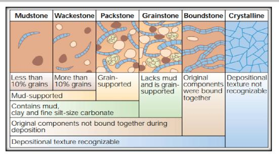
Figure 2. Dunham Classification for carbonate rocks (After Dunham, 1962).
