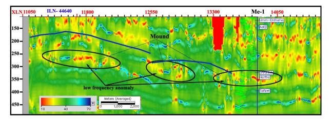
Figure 10.3-D seismic in-line section shows the low instantaneous frequency through mound seismic facies in the Hartha formation.
